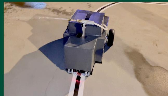
Figure 3: The device following a predetermined line and spraying water.
